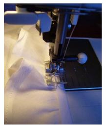
Sewing binding to ruffle seam.
